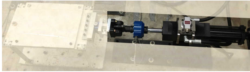
Figure 1.6: Servo-hydraulic actuator as a common transfer system.
